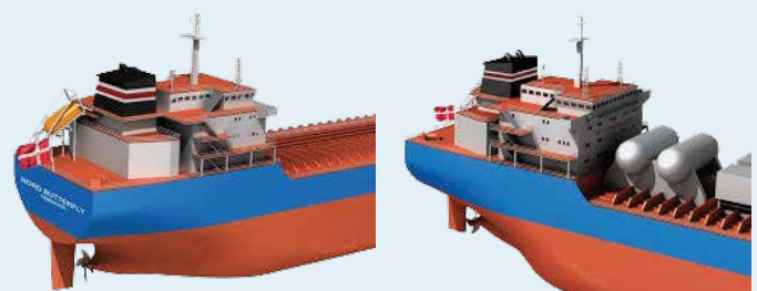
Aft Ship with Scrubber installed having enlarged funnel and LNG tank on the main deck
