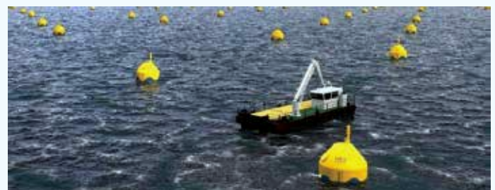
In wave energy technology, the movement of a buoy induced by waves flowing from all directions generates energy relative to the base connection
