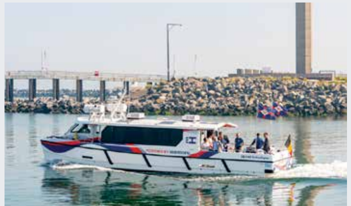
Hydroville uses hydrogen gas as its fuel
